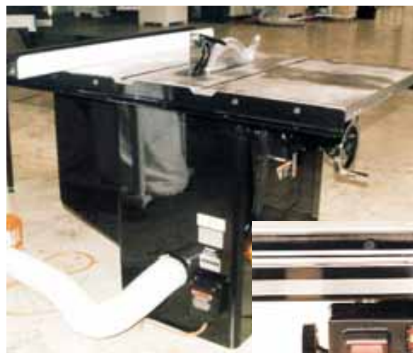
Photo.3: Dust connection at the rear
