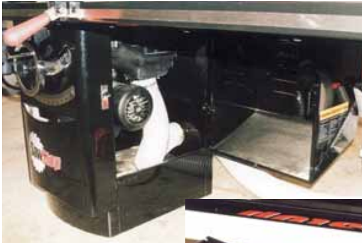
Photo.4: Large access doors on both sides of the cabinet housing are a welcome feature
