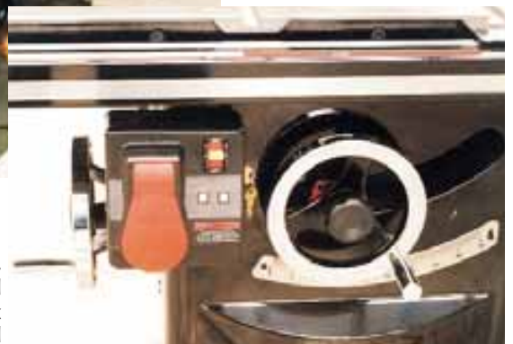
Photo.2: From left to right, the rise and fall handwheel, control box and tilt handwheel
