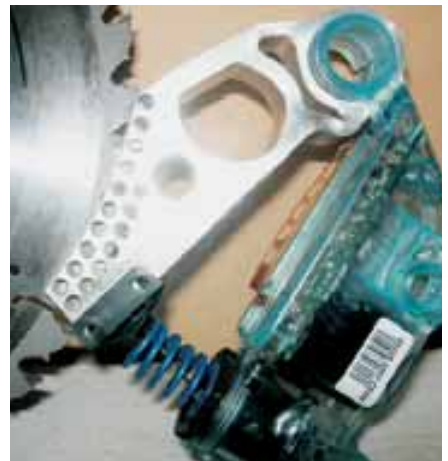
Photo.7: A 'used' cartridge. The charge releases the spring which then rams the aluminium block into the blade. The distortion around the pivot point is intentional as it absorbs some of the centrifugal force of the blade
