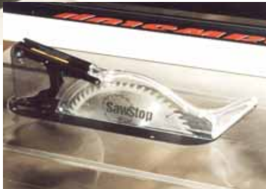
Photo.5: Low profile transparent blade guard attached to a quick-change mount
