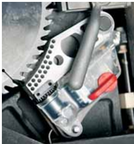
Photo.6: The SawStop cartridge in position
